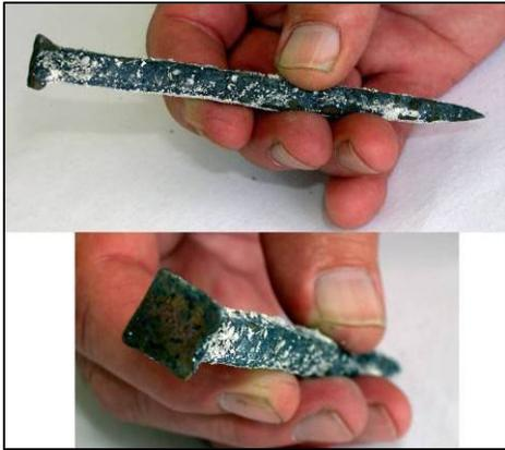
The dump bolt was driven into the wood for additional stability in conjunction with fasteners that extended through the planks into the frames. The dump bolt did not go through the full timber.
