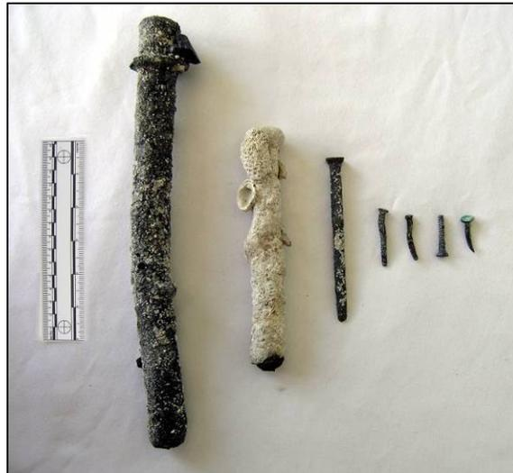
Fasteners from left: Copper-alloy driftbolt, iron driftbolt, dump bolt, iron nail, iron nail, screw, copper-alloy sheathing nail.
