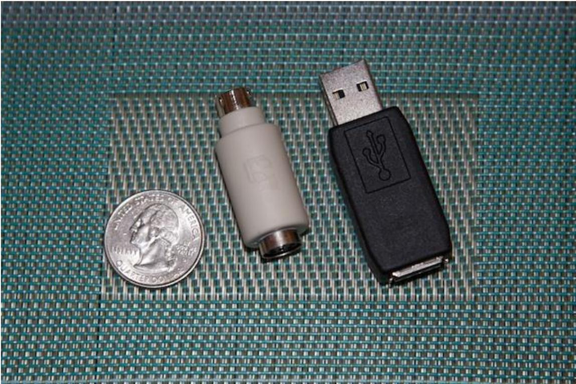
Keylogging devices cannot be detected by software, and must be discovered via physical inspection. It is important to regularly inspect patron computers for foreign devices. Any suspicious activity associated with the cabling areas of the computers should be noted and investigated. It would be logical for criminals to use minors to place and retrieve keylogger devices.
