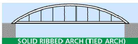
Some metal bridges which appear to be open spandrel deck arch are, in fact, **cantilever**; these rely on diagonal bracing. A true arch bridge relies on vertical members to transmit the load which is carried by the arch.
