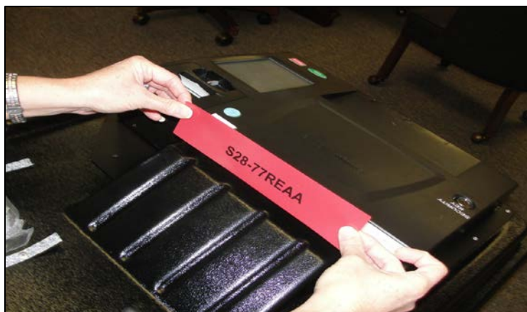
Figure 7 - Security seal as applied over chute of ICP (340C) ballot box
