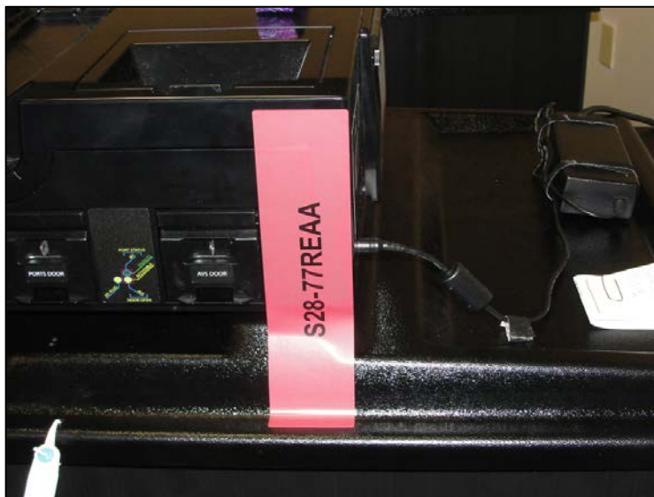
Figure 23 - Security seal attaching ICE (420A) box to the right side of the ICE tabulator
