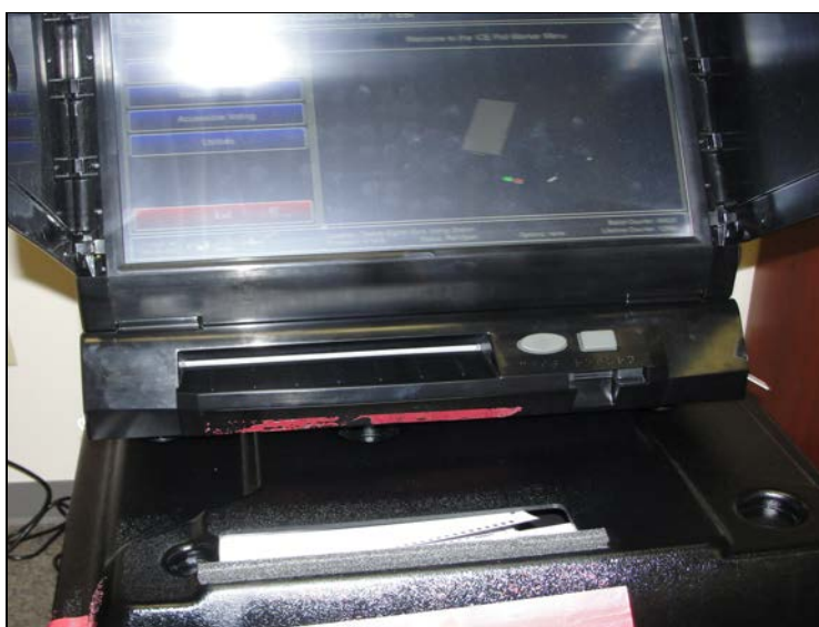
Figure 25 - Security seal residue on ICE tabulator
