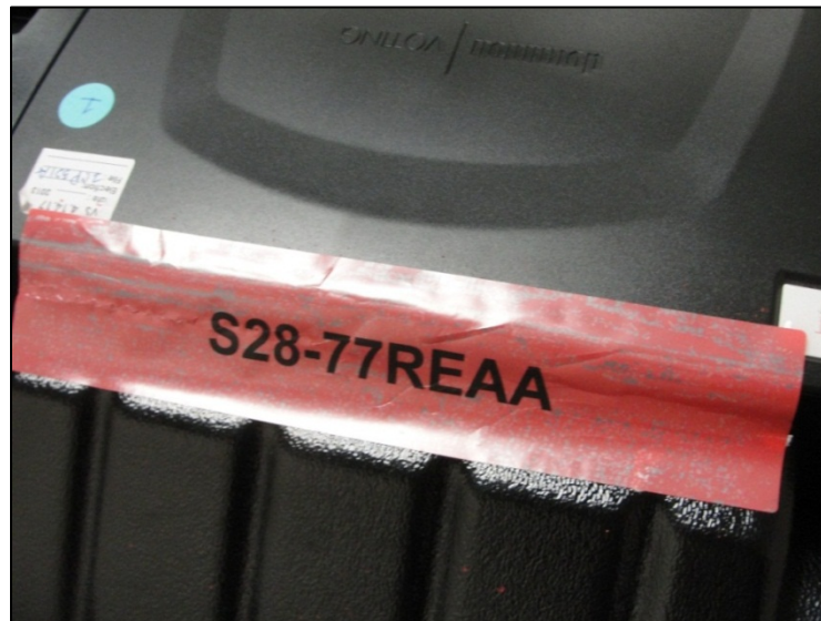
Figure 12 - ICP tabulator showing evidence of tampering
