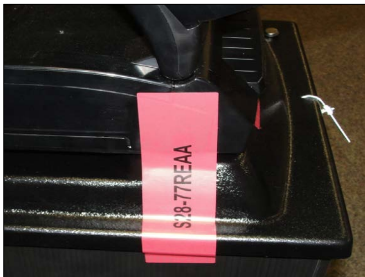
Figure 22 - Security seal attaching ICE (420A) ballot box to the left side of the ICE tabulator
