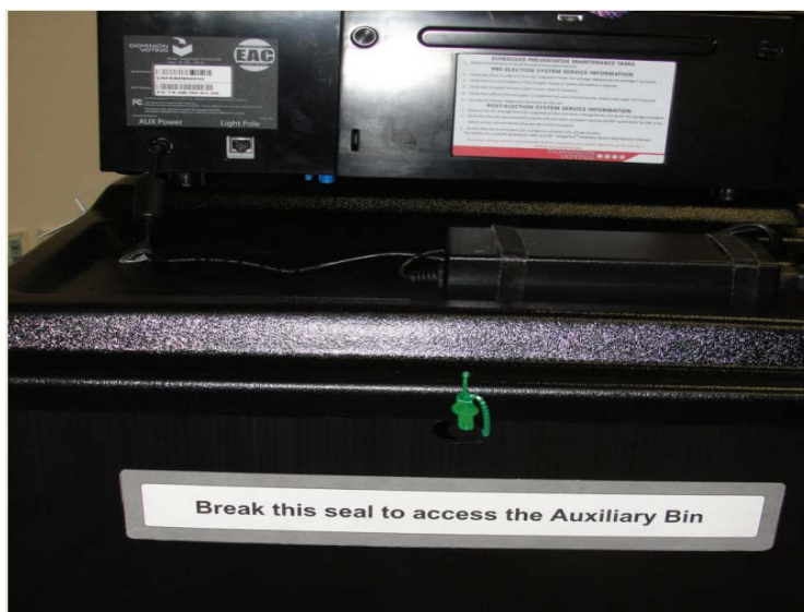
Figure 20 - Security seal applied over auxiliary bin slot of ICE (420A) ballot box
