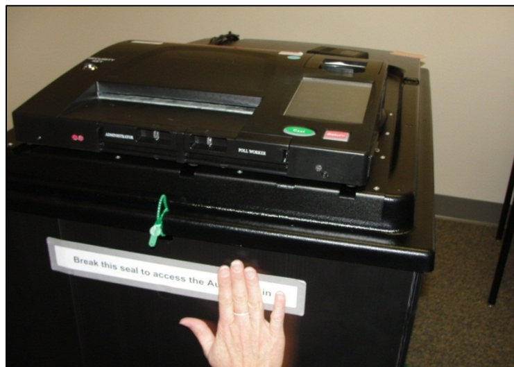
Figure 8 - Security seal as applied over auxiliary bin slot of ICP (340C) ballot box
