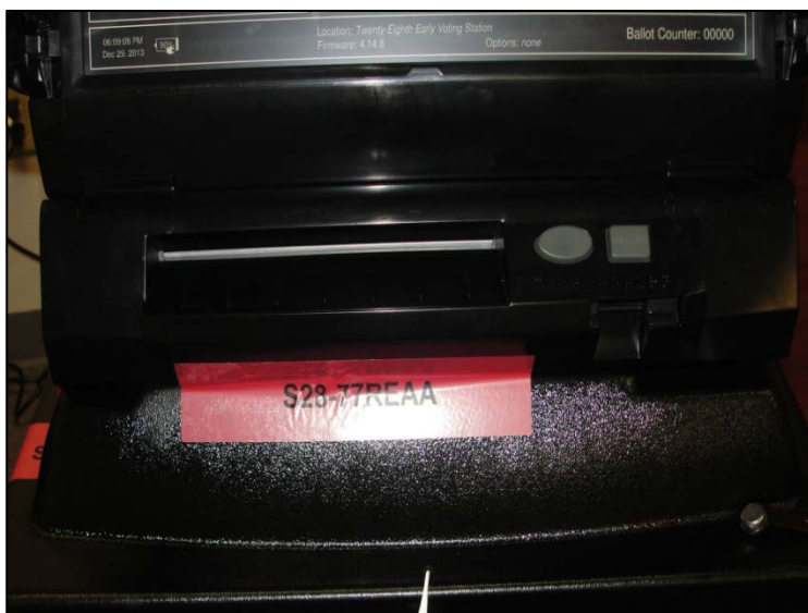
Figure 21 - Security seal attaching ICE (420A) ballot box to the front of the ICE tabulator
