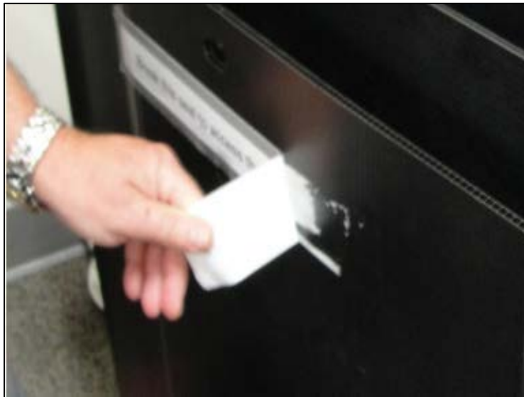
Figure 10 - Auxiliary security seal residue on ICP (340C) ballot box
