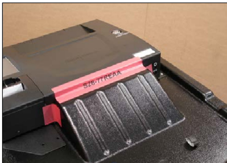
Figure 9 - Security seals applied to the top and sides of ICP (340C) ballot box chute
