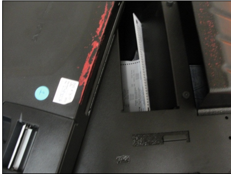
Figure 11 - Security seal residue on ICP tabulator
