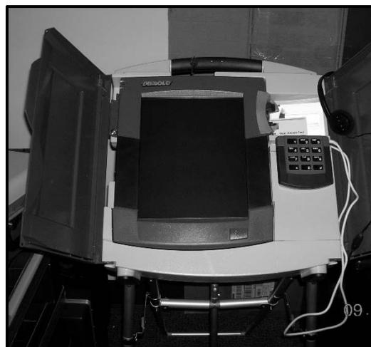
Figure 2. AccuVote TSx direct recording electronic device
