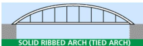
Some metal bridges which appear to be open spandrel deck arch are, in fact, **cantilever**; these rely on diagonal bracing. A true arch bridge relies on vertical members to transmit the load which is carried by the arch.
