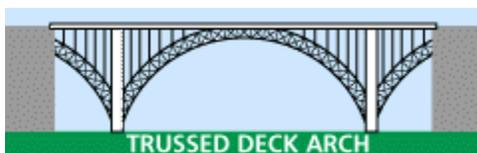
The tied arch (bowstring) type is commonly used for **suspension** bridges; the arch may be trussed or solid. The trusses which comprise the arch will vary in configuration, but commonly use Pratt or Warren webbing. While a typical arch bridge passes its load to bearings at its abutment; a tied arch resists spreading (drift) at its bearings by using the deck as a tie piece.
