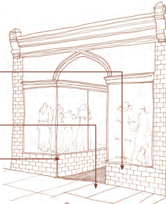
The metal frames flanking the window and door openings are used to hold flood barriers in place.
